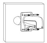
③ Tie the safety rope to hook and thread the cable
